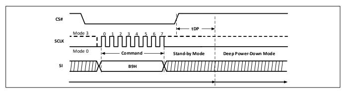
Figure-22. Deep Power-Down Sequence Diagram
