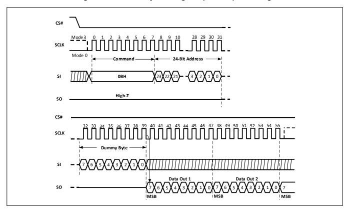
Figure-8. Read Data Bytes at Higher Speed Sequence Diagram
