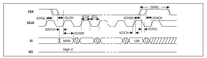
Figure-33. Output Timing
