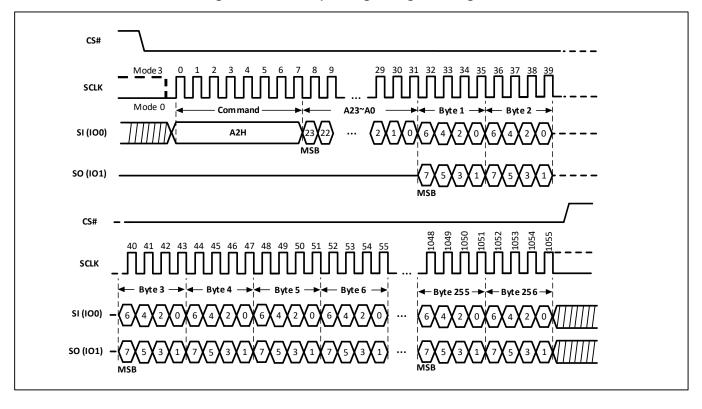
Figure-18. Dual Input Page Program Diagram
