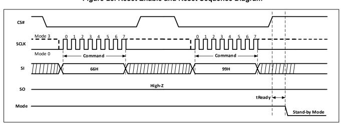
Figure-28. Reset Enable and Reset Sequence Diagram
