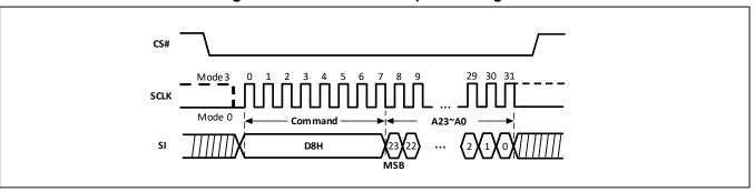
Figure-15. Block Erase Sequence Diagram
