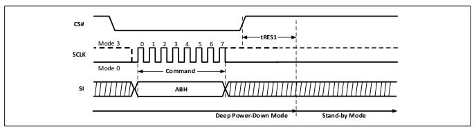
Figure-23. Release from Deep Power-Down (RDP) Sequence Diagram
