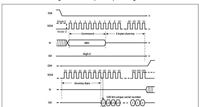
Figure-29. Read Unique ID Sequence Diagram
