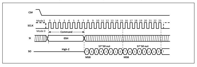
Figure-5. Read Status Register Sequence Diagram
