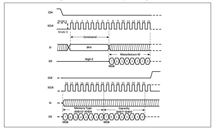
Figure-27. Read Identification Sequence Diagram
