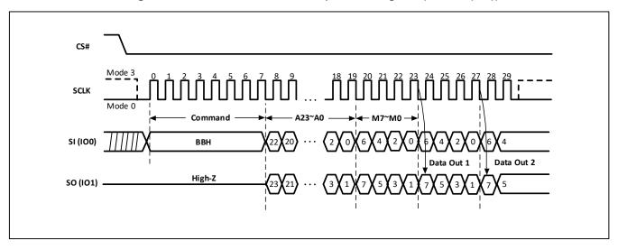
Figure-10. Dual I/O Fast Read Sequence Diagram (M5-4  $\neq$  (1,0))
