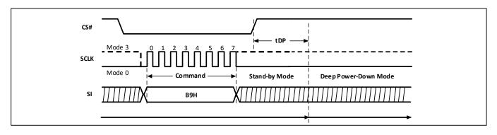
Figure-21. Deep Power-Down Sequence Diagram
