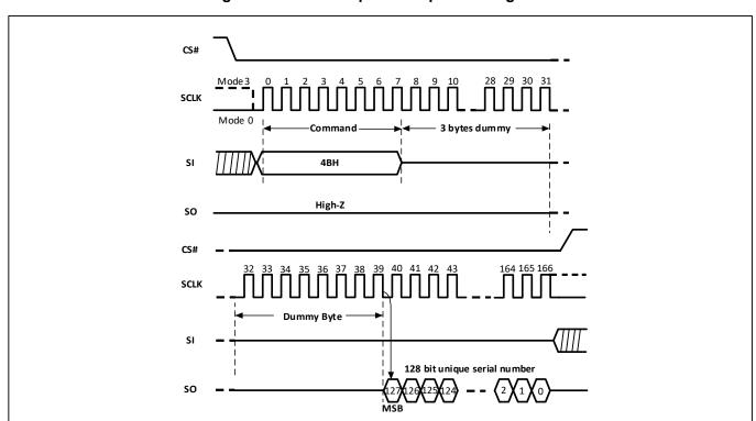
Figure-28. Read Unique ID Sequence Diagram
