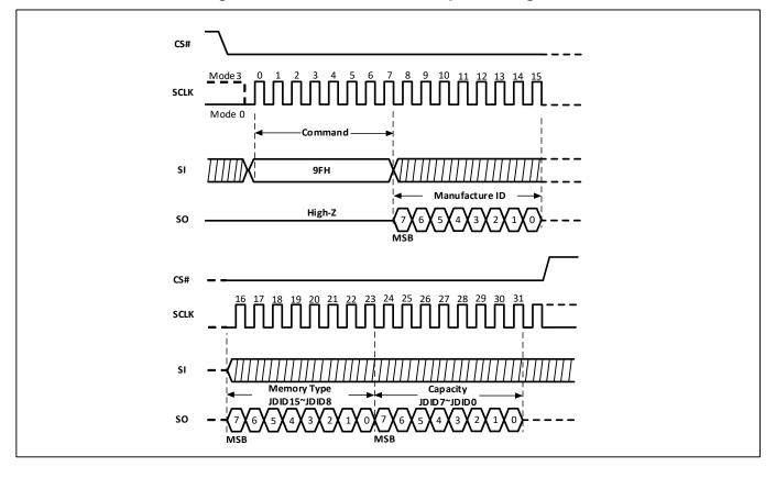
Figure-26. Read Identification Sequence Diagram
