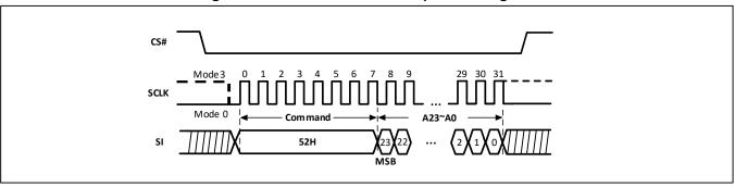
Figure-14. Half Block Erase Sequence Diagram
