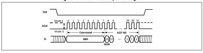
Figure-15. Block Erase Sequence Diagram
