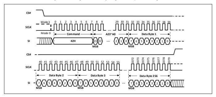
Figure-19. Program Security Register Sequence Diagram
