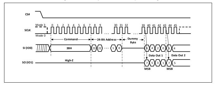
Figure-9. Dual Output Fast Read Sequence Diagram
