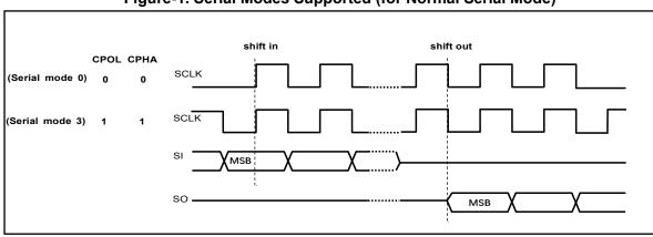
Figure-1. Serial Modes Supported (for Normal Serial Mode)
