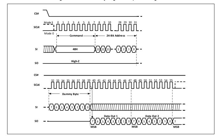
Figure-20. Read Security Register Sequence Diagram
