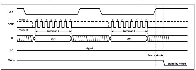
Figure-27. Reset Enable and Reset Sequence Diagram
