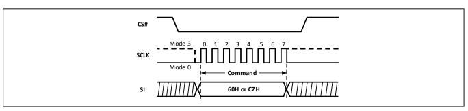
Figure-16. Chip Erase Sequence Diagram
